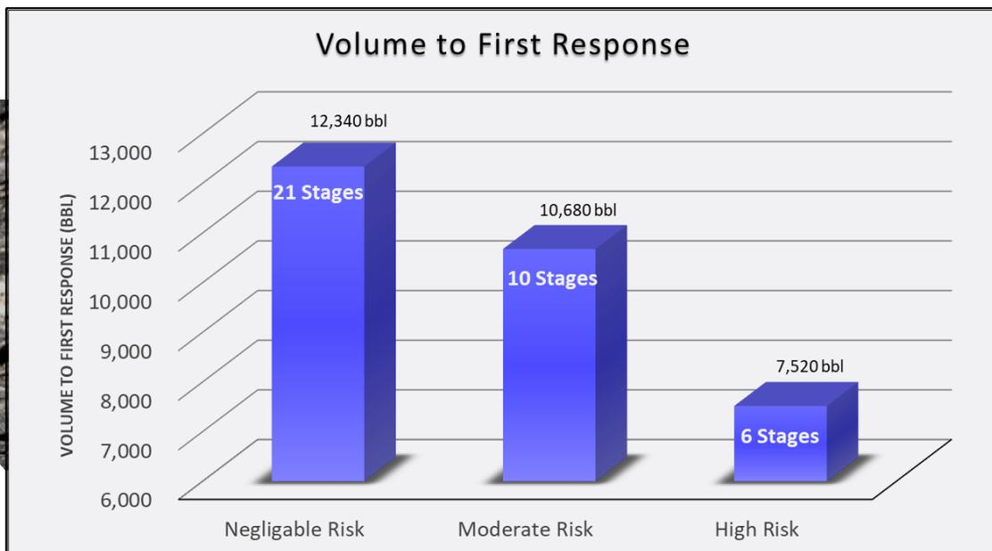
Volume to first response in offset well measured by fiber optics compared to fracture risk as identified by Drill2Frac.
